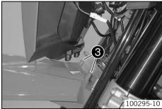
Remove the cloth from the fender, attach the headlight mask to points 3 on the fender and swing it up to the steering head.
