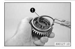
Extract the lock ring • from the groove using suitable pliers.
