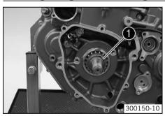
Heat the timing chain sprocket and push it immediately on to the crankshaft.
