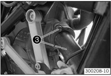
Remove nuts **3** of the manifold.
