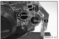
Attach the water pump wheel ②. Mount and tighten screw ③
