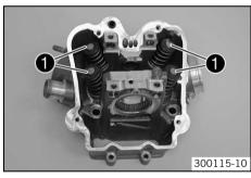
Take the shims **1** out of the valve spring retainers and lay them to one side according to their normal built-in position.
