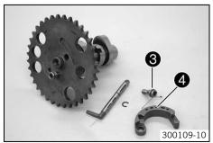
Disconnect the autodecompression spring. Loosen the screw 3 and remove it together with the autodecompression spring and the autodecompression weight 4.
