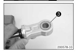
Remove seal rings 3 on both sides.
