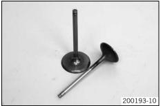
Check the run-out at the valve plate.
