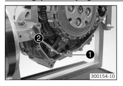
Remove the spacer • and spring • of the shift shaft.
