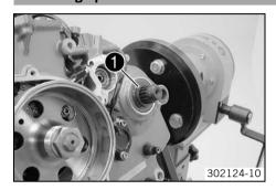
Remove the spacer • of the countershaft.
