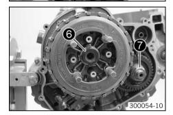
Hold the clutch cage using the special tool and remove the nut 3 of the inner clutch hub.
