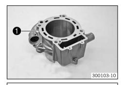
Check the sealing area of the cylinder head for distortion using a straight edge and the special tool.
