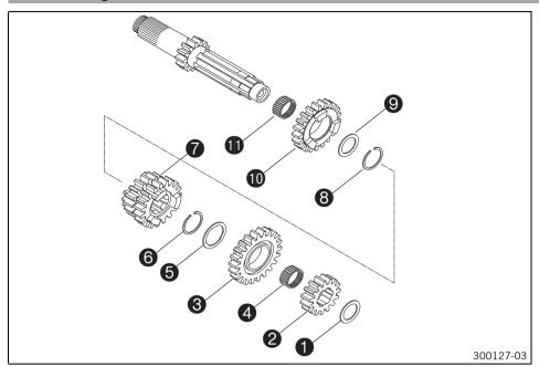
Fix the main shaft in the vise with the geared end facing downward.
