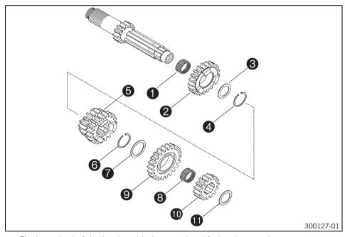
Fix the main shaft in the vise with the geared end facing downward.
