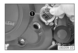
Remove the oil filler plug with O-ring • from the clutch cover and fill up with engine oil.
