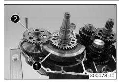
Remove the crankshaft • and the balancer shaft •.
