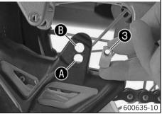
Remove screws • and •. Take off the chain guide.
