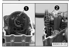
Remove screw ①. Take off the camshaft support plate ②.
