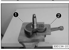
Fix the crankshaft with special tools 1 and 2 in the vise.
