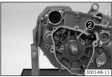
Thread the timing chain ② in and lay it over the timing chain sprocket.
