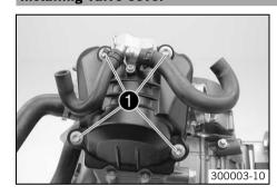
Put the valve cover in place with the seal. Mount and tighten screws ①.
