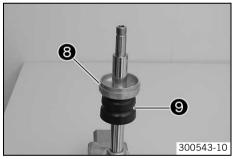
Remove locking cap 3 and rubber buffer 9.
