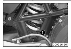
The shock absorber part number • is on the right of the shock absorber.
