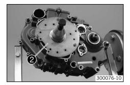
Install the special tool ② with suitable screws.
