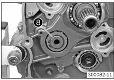
Install the shim 3 and lock ring of the countershaft.
