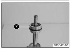
Remove seal ring retainer **7**.
