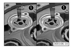
Use a feeler gauge • to measure the play between the external rotor and the engine case as well as between the external rotor and the internal rotor.
