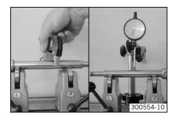
Measure the diameter of the piston rod.
