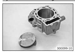
**Nikasil®** is a surface protection layer for a coating method developed by the Mahle company. The name is derived from the two materials used in this method - a layer of nickel, in which silicon carbide (a particularly hard substance) is embedded. The most important advantages of the **Nikasil®** coating are the excellent heat conductivity resulting in better performance, less wear, and low cylinder weight.
