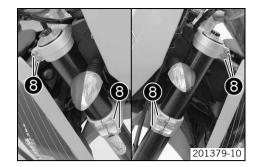
Loosen the screws 3 of the triple clamp. Remove the fork legs from the bottom.
