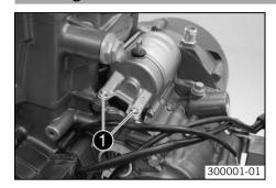
Grease O-ring. Mount the starter motor.
