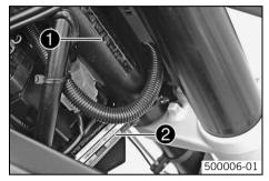
The chassis number **1** is stamped on the right of the steering head. The USA type label **2** is on the right of the frame behind the steering head.
