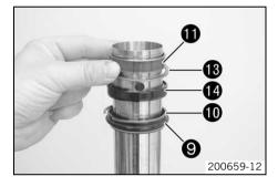
Heat up the outer tube in area • of the lower sliding bushings.
