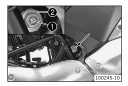
Turn the adjusting screw ① clockwise with a screwdriver up to the last perceptible click.
