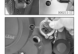
Remove the oil filler plug with O-ring from the clutch cover and fill up with engine oil.
