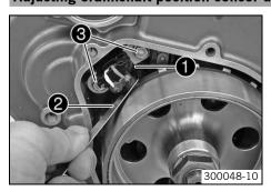
Adjust the distance between the crankshaft position sensor • and the conductive element of the rotor using the special tool 2.
