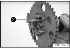
Pull the autodecompression shaft **2** from the camshaft.
