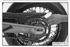
Push the rear wheel forwards as far as possible and take the chain off the rear sprocket.
