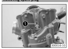
Remove the spark plug using the special tool 1.
