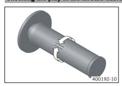
Move the handlebar to the straight-ahead position. Move the throttle grip backwards and forwards to ascertain the play in the throttle cable.
