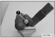
Remove compression damping adjuster •. Remove the spring, sleeve and piston.
