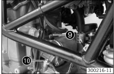
Position the electrical connection • on the starter motor. Mount and tighten screw.
