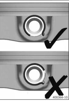
Position the piston pin retainer.
