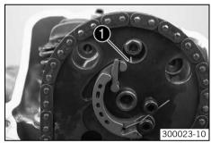
Turn the crankshaft counterclockwise until markings • of the camshafts are flush with the marks of the camshaft support plate.
