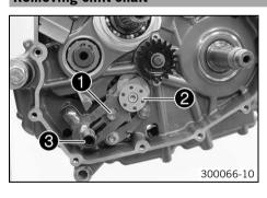
Push sliding plate 1 away from the shift drum locating 2. Remove shift shaft 3 with the washer.
