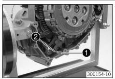
Install the spacer • and spring • of the shift shaft.
