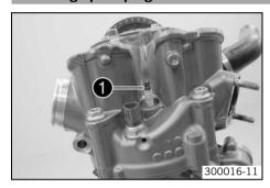
Mount and tighten the spark plug • using the special tool.
