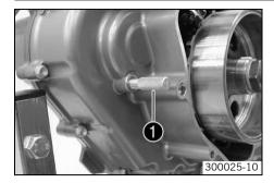
Set the crankshaft to top dead center and lock it with the special tool ①.
