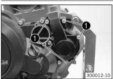
Remove screws ①. Take off the water pump cover.
