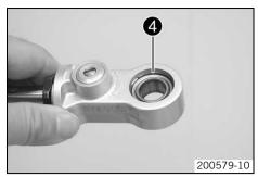
Remove lock rings 4 on both sides.
