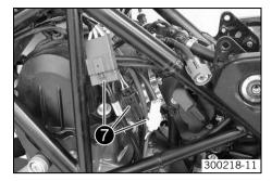
Reconnect plug connectors of the gear position sensor, the crankshaft position sensor and the alternator.
