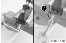
Loosen screw of the cartridge and remove it with the sealing ring.
