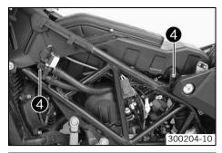
Mount and tighten screws 4.
