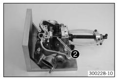
Remove the small camshaft bearing ② using the special tool.
