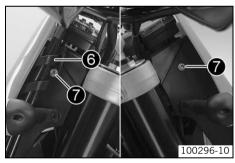
Position brake-hose guide **6**. Mount and tighten screws **7**.
