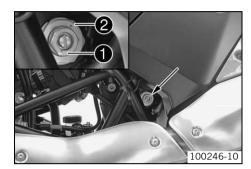
Turn adjusting screw 1 all the way clockwise using a socket wrench.
