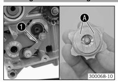
Press locking lever **1** down and position shift drum locating.
