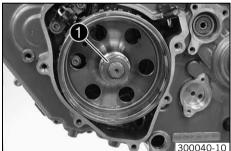
Use the special tool to hold the rotor tight.
