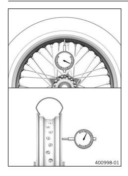
Check the axial run-out and radial run-out of the rim.
