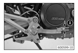
Move the foot brake lever back and forth between the end stop and the contact to the foot brake cylinder piston and check free travel .
