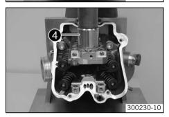
Press in the large camshaft bearing as far as possible using the special tool 4.
