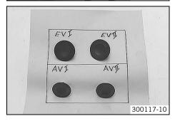
Place the valve into a box according to the installation position and label the
