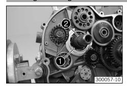
Install supporting plate • and needle bearing •.
