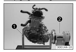
Mount special tool • on engine work stand •.
