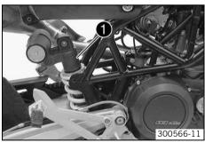
Swing the rear end upwards and insert shock absorber • from above.
