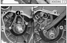
Position the timing chain securing guide 1.
