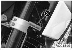
The Canada type label 3 is on the right of the frame behind the steering head.
