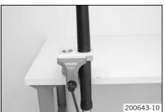
Clamp the fork leg in the area of the lower triple clamp.
