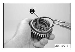
Insert the lock ring (a) into the groove with suitable pliers and check that it is seated correctly.
