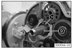
Remove needle bearing 9 and supporting plate 0.
