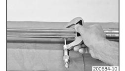
Measure the external diameter of the inner tube in several places.
