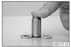
Place two spacing washers or similar aids next to the piston of the timing chain tensioner. This should ensure that when pushed down, the piston does not fully withdraw.
