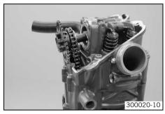
Pull the camshaft out of the bearing seats. Take the timing chain off the camshaft gear. Remove the camshaft.
