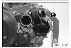
Put on the water pump cover **⑤**. Mount and tighten screws.
