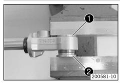
Place special tool • underneath and press in the heim joint as far as the center using special tool •.
