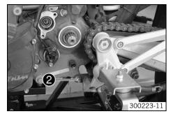
Install the screw and nut ② of the lower engine bracket, but do not tighten them yet.
