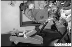
Remove the floor jack with the special tool.
