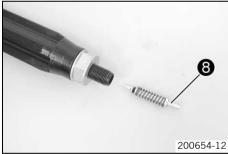
Remove valve 3 of the rebound damping with the spring from the cartridge.
