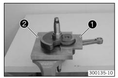
Fix the crankshaft with special tools • and • in the vise.
