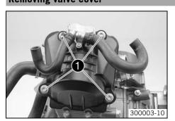
Remove screws ①. Take off the valve cover with the valve cover seal.
