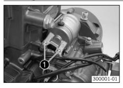
Remove screws 1. Take off the starter motor.
