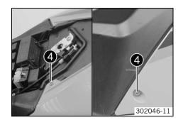
Mount and tighten screws **4**.
