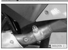
Position the manifold at the rear with the seals.
