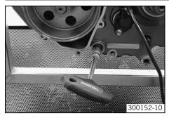
Push the oil screen with O-rings on to a pin wrench. Push the pin wrench through
