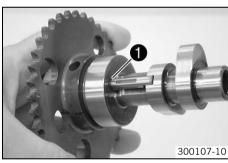
Take the lock ring • off the autodecompression shaft and dispose of it.
