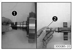
Mount the special tool • on the alternator side of the crankshaft.
