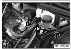
Loosen the spring-loaded band-type clamp from the breather, SLS and oil return line with the special tool.
