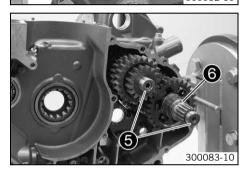
Pull both transmission shafts **6** out of the bearing seats together.
