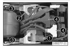
Slide the battery into the battery rack.
