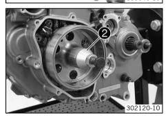
Install the special tool ② on the rotor. Hold it tight using the special tool and pull
