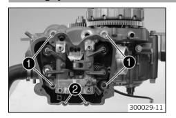
Put on the cylinder head gasket.
