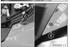
Mount and tighten screws 6.
